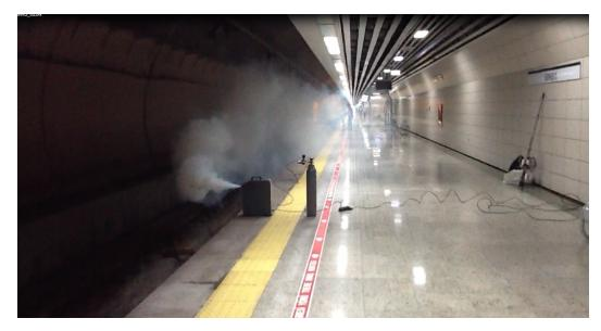
Figure 1.13: Smoke Test in Sirkeci Metro Station
