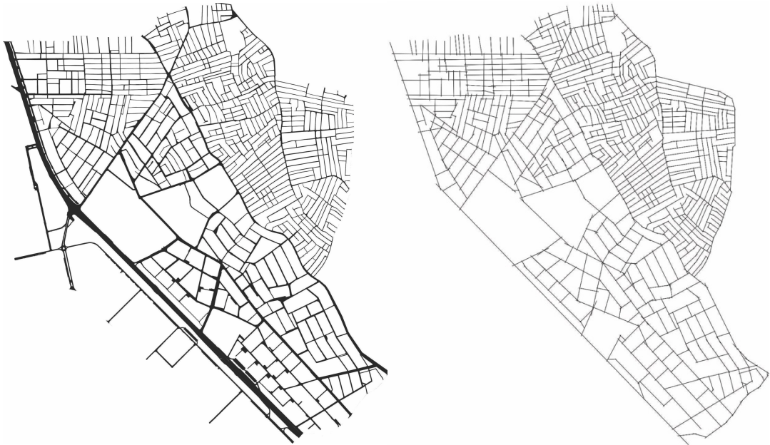
Figure 4.26: Street pattern of the site (left), and the axial map drawn from the actual layout (right)
