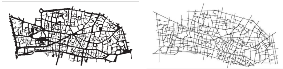
Figure 4.25: Illustration of public open spaces of the City of London (left), and axial map of the City of London (right), (Source: Hillier, 2007, p.117)
