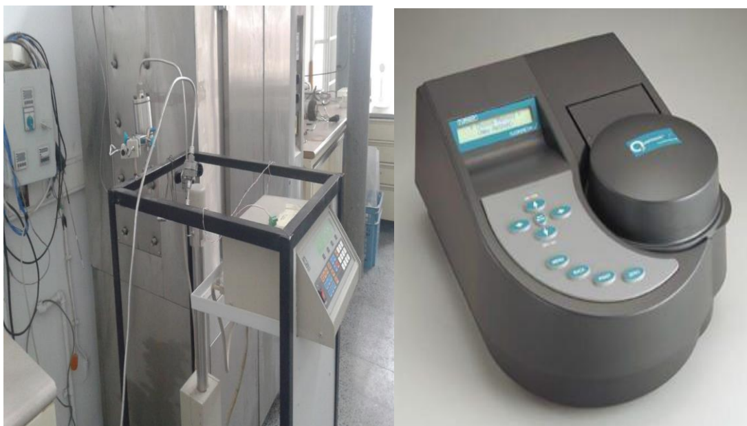
Figure 4.5. 260D Syringe Pump and The Turner Quantech Digital Filter Fluorometer
