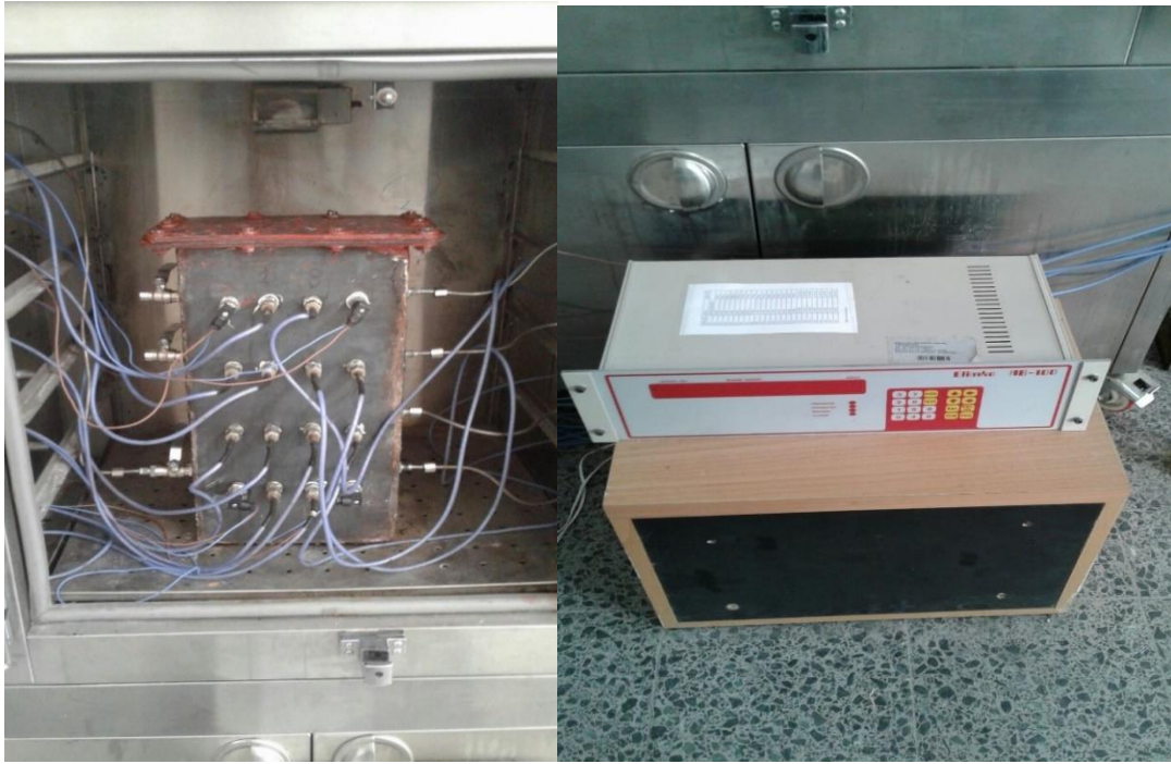
Figure 4.4 Thermocouples, Pressure Transducer and Scanner
