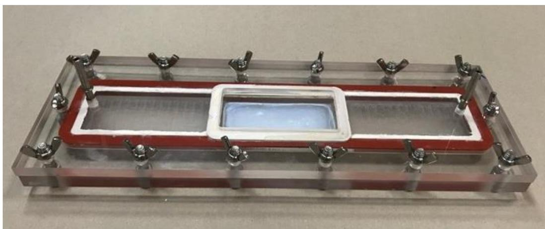
**Figure B.1** The photoreactor used in photocatalytic NO Oxidation experiments
