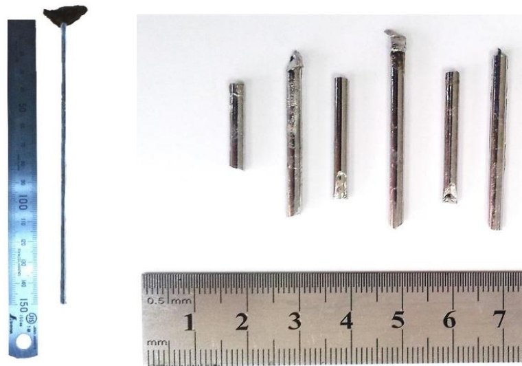
Figure 4.6. M_{60}Cr_{13}Mo_{10}B_8Y_2Mn_7 samples fabricated by suction casting
