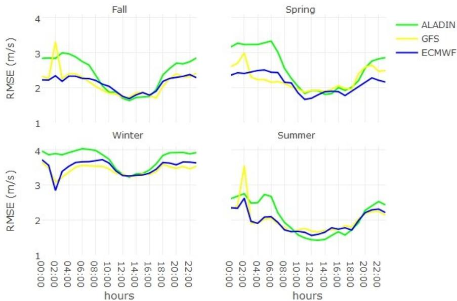
Figure 3.25 Diurnal Cycles for RMSE of Wind Speed (WPP-2)
