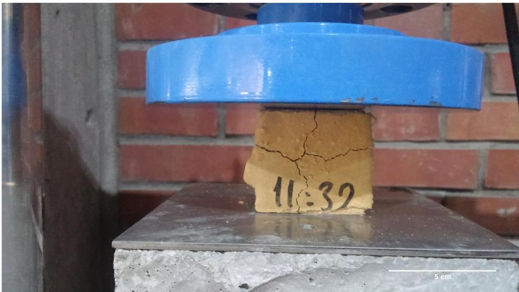
Figure C.1 Cracks on the 5-cm cube sample with  $M/P = 6$  and  $W/B = 0.20$  at 24 h (before testing)
