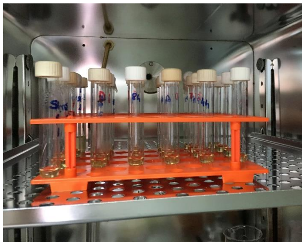
Figure 4.20. Photograph of time kill test samples in incubator.
