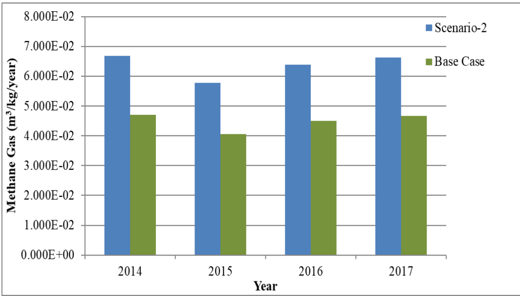
Figure 31. Comparison of scenario-2 and base case (mixed waste with 56% organic content) for LandGEM
