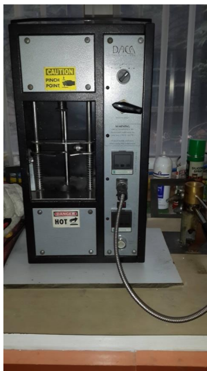
Figure 3.5 The laboratory scale injection-molding machine.
