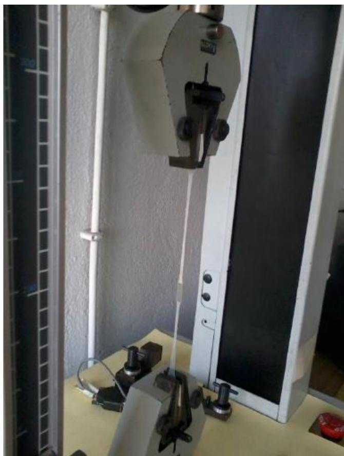
Figure 3.3 The photograph of tensile test machine used in this study.
