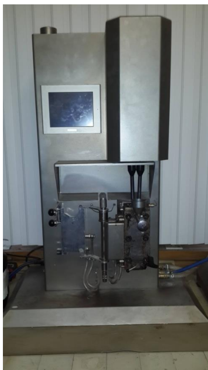
Figure 3.4 The twin screw extruder used in this study for the production of blends.
