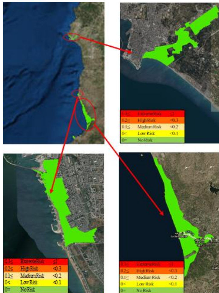
Figure 4.13 Normalized economic risk maps for Latakia City Center (top right), Tartus City Center (bottom left) and Tartus Agricultural Area (bottom right) in Syria
