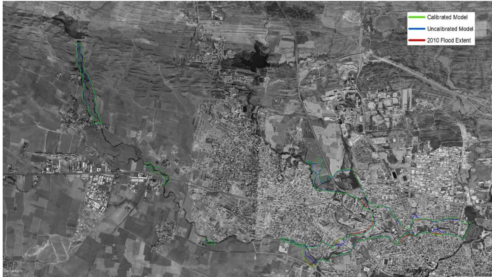
Figure 7.7. The boundaries of maximum flood extent maps of 2010 flood event (red line), calibrated model (green line), and uncalibrated model (blue line)
