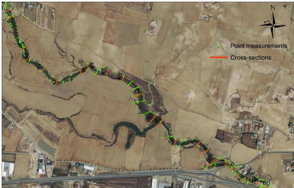
Figure 4.8. Surveying of cross-sections
