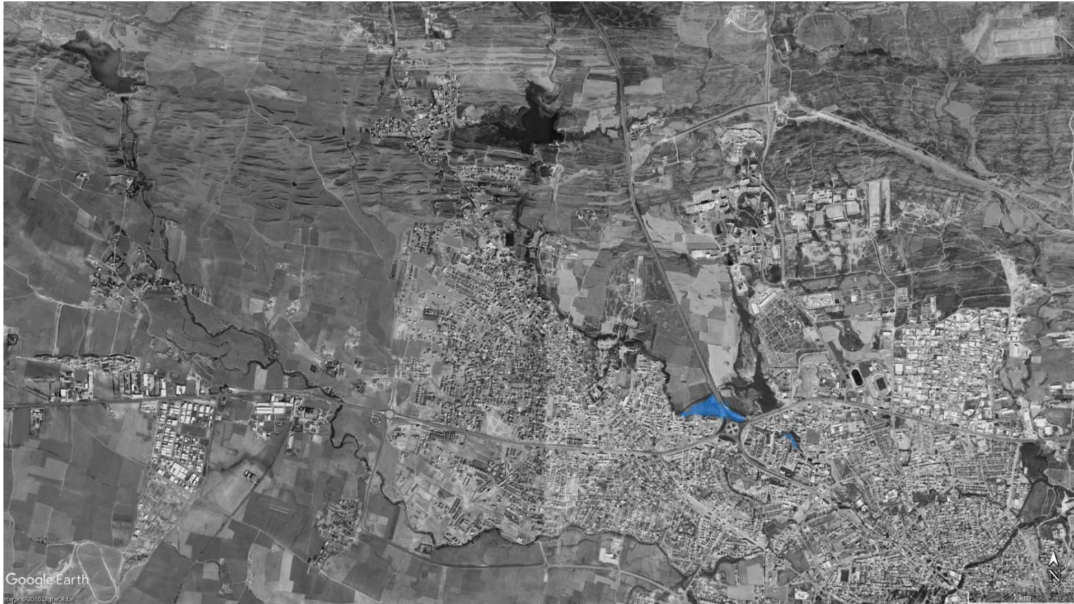
Figure 7.25. Flood extend obtained by applying the final solution of Kanlıköy and Gönyeli ponds with reasonably smaller Manning's coefficient
