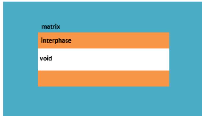
Figure 6.2 – Side view of considered geometry for the FE model in Malagu et al. (2017) (not to scale)
