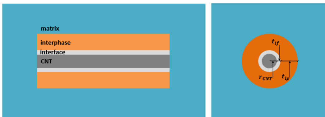
Figure 6.1 – Side and cross section views of considered geometry for the MD model in Malagu et al. (2017) (not to scale)
