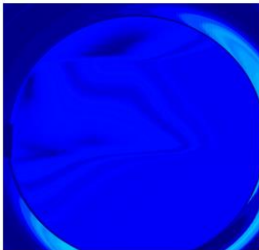
Figure 74. c-SAM image of the bonded pair at 10 \mu\text{m} resolution.
