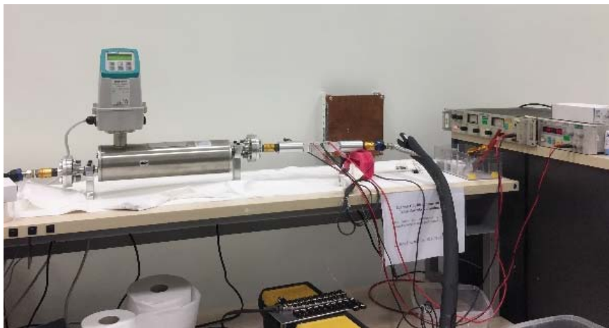
Figure 3.8: Experimental setup with power supplies before insulation application
