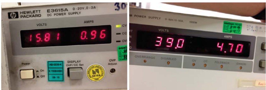
Figure 3.13: Power supply settings of the diamond resistors with 5 W heat dissipation (left) and 30 W heat dissipation (right)
