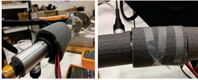
Figure 3.9: Insulation of module and pressure transmitter adaptors
