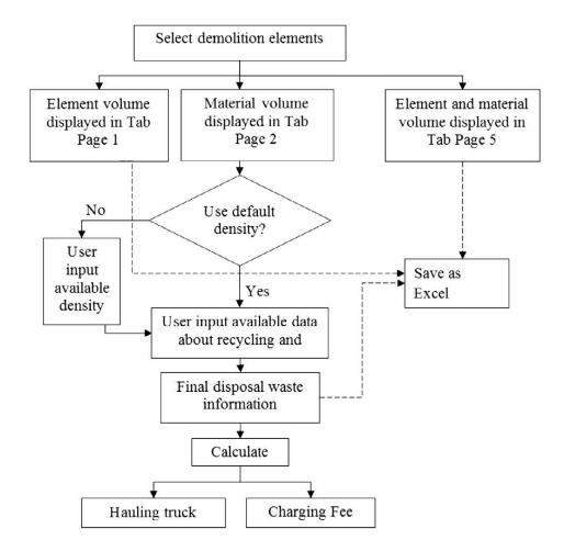
Figure 1-2: BIM-based demolition waste estimating system operation flowchart
