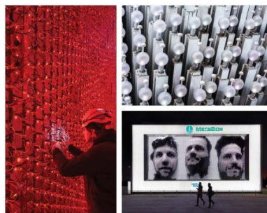
Figure 3.2. Megafaces Pavillion, The world's first 3d actuated large-scale LED screen, 2014, Asif Khan
