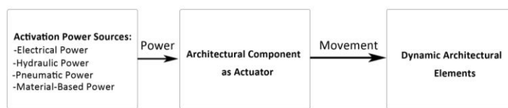
Figure 3.1.Activation Power Forces of Actuators
