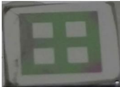
Figure 31. Crystal named MT13-RX1-W39 after photolithography is finished.
