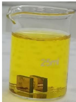
Figure 32. Electroless deposition in action for samples named as MT13-RX1-W34 and MT13-RX1-W35.
