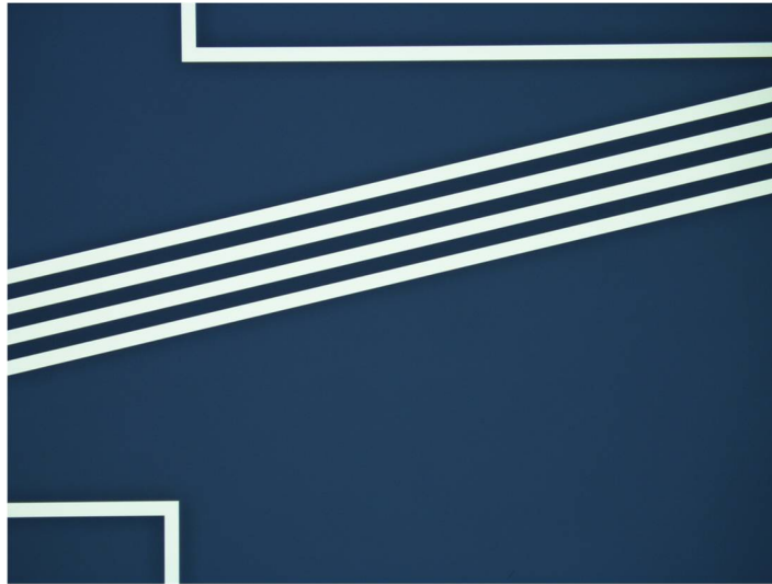
Figure 4.13. The image of the planar electrodes after wet metal etching step
