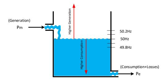
Figure 2.1: Frequency Behaviour in Electric Grid with the Water Level in a Container Analogy [30]
