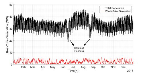
Figure 5.13: Variation of the Total and Solar+Wind Energy Production between 01 Jan. 2018 and 31 Dec. 2018 (hourly basis) [35]
