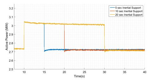
Figure 4.13: Active Power Output of the Wind Turbine for High Wind Scenario
