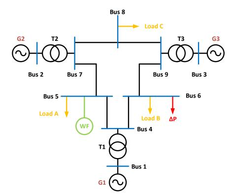
Figure 5.5: 10% Renewable Generation Case Single Line Diagram
