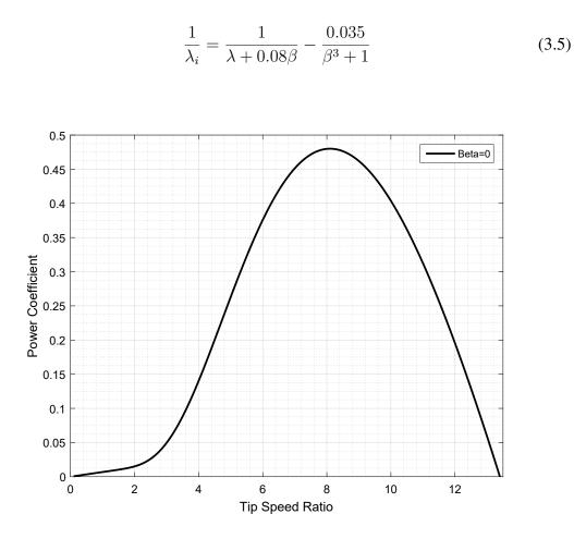
Figure 3.2: Power Coefficient Variation with Tip Speed Ratio under Zero Pitch Angle
