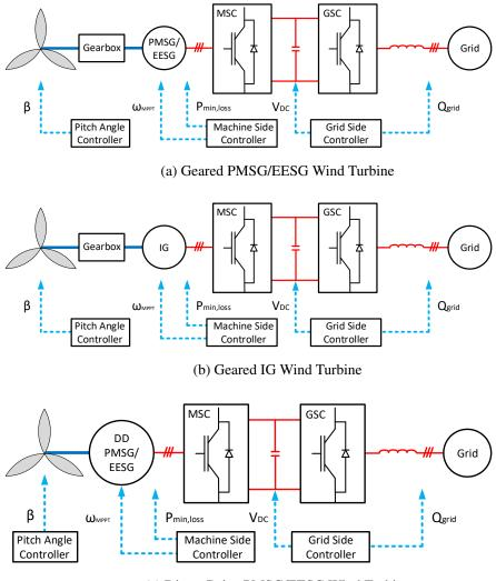
(c) Direct-Drive PMSG/EESG Wind Turbine
