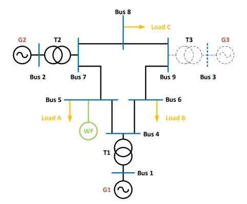
Figure 5.7: Reduced Inertia Case Single Line Diagram
