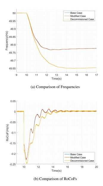
Figure 5.8: Comparison of Base Case, 10% Renewable Generation Case (Modified Case) and Reduced Inertia Case (Decommissioned Case)
