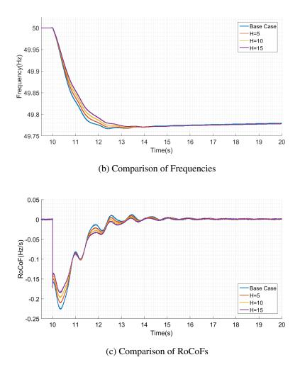
Figure 5.9: Emulation of the Different Inertia Constants in the 10% Renewable Generation Case
