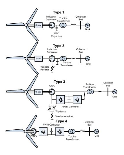
Figure 1.4: Wind Turbine Generator Configurations [12]
