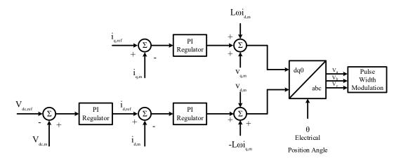
Figure 3.8: Grid Side Controller Diagram
