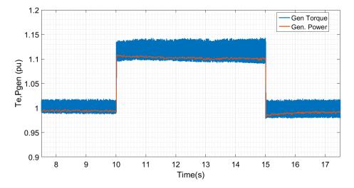
Figure 4.10: Fast Inertial Support Active Power Limit for High Wind Scenario
