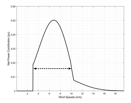
Figure 4.6: Distribution of Fast Inertial Support
