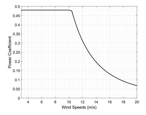
Figure 3.5: Power Coefficient Variation for GE 2.75-103
