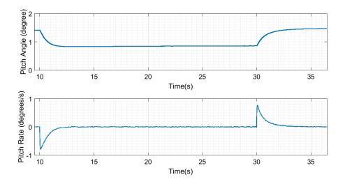
Figure 4.15: Pitch Angle and Rate of Change of Pitch Angle for High Wind Scenario for 20 Seconds Support
