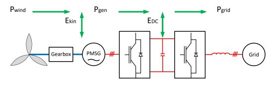
Figure 4.1: Active Power Flow Diagram
