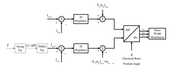
Figure 3.10: Modified MSC for Inertial Support
