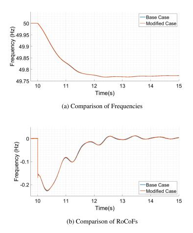
Figure 5.6: Comparison of Base Case and 10% Renewable Generation Case
