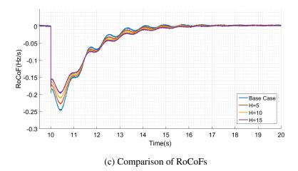
Figure 5.10: Emulation of the Different Inertia Constants in the Reduced Inertia Case
