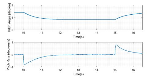
Figure 4.12: Pitch Angle and Rate of Change of Pitch Angle for High Wind Limit Scenario
