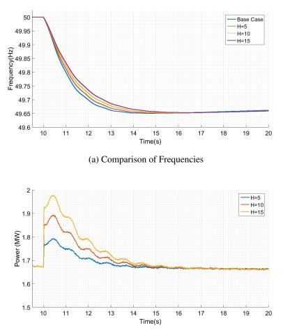
(b) Active Power Generations of the Wind Farms (wind speed=9m/s and n=1490rpm)
