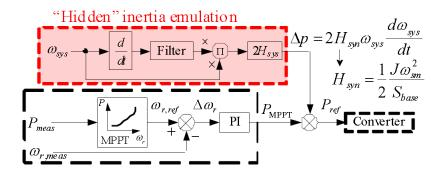
Figure 1.6: Hidden Inertia Controller in [24]
