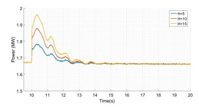
(a) Active Power Generations of the Wind Farms (wind speed=9m/s and n=1490rpm)
