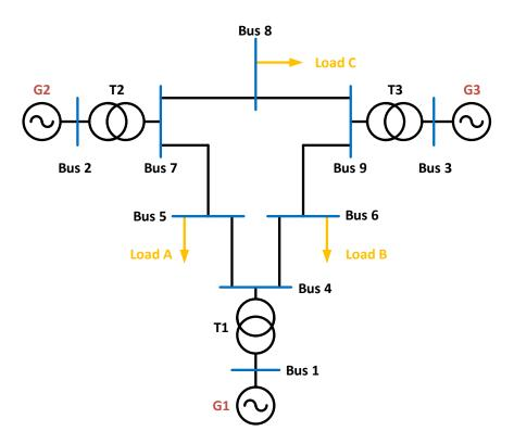
Figure 5.1: P.M. Anderson Test Case [59]
