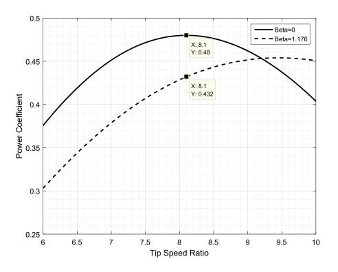
Figure 3.3: Power Coefficient Variation for Two Different Pitch Angle
