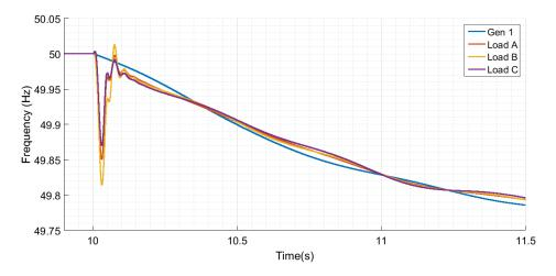
Figure 5.4: Frequencies in Generator 1 and Load Buses
