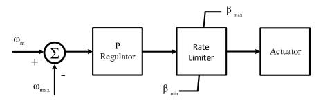
Figure 3.4: Pitch Angle Control Diagram
