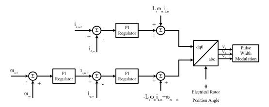
Figure 3.7: Machine Side Controller Diagram
