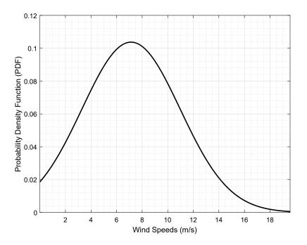
Figure 4.5: Probability Density Function of Measured Wind Speeds
