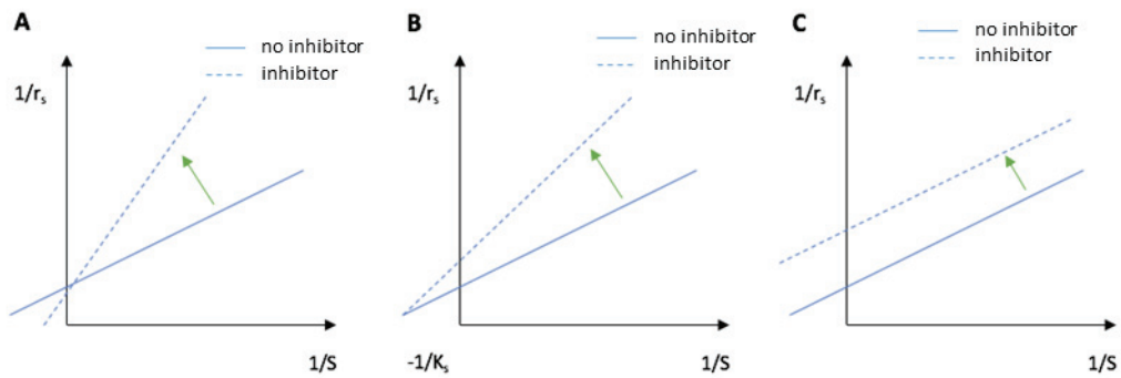
Figure 3 Lineweaver-Burk Representations Competitive (A), Non-Competitive (B) and Un-Competitive (C) Inhibition (Henze et al., 2008)
