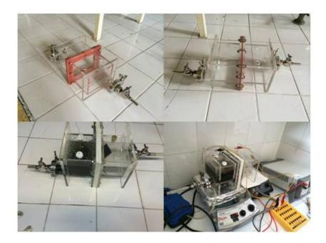
Figure 3.2. Dual chamber MFC reactor configuration and set-up details
