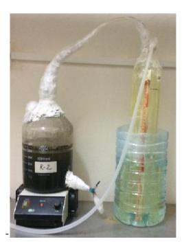
Figure 3.3. Reactor set-up including the gas collection unit
