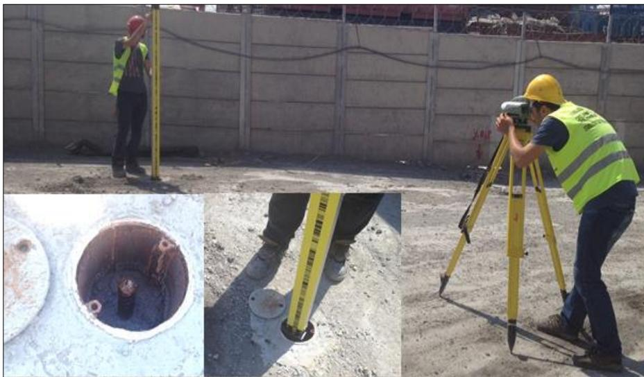
Figure 3.8. Ground settlement bolts and taking measurement in the study area
