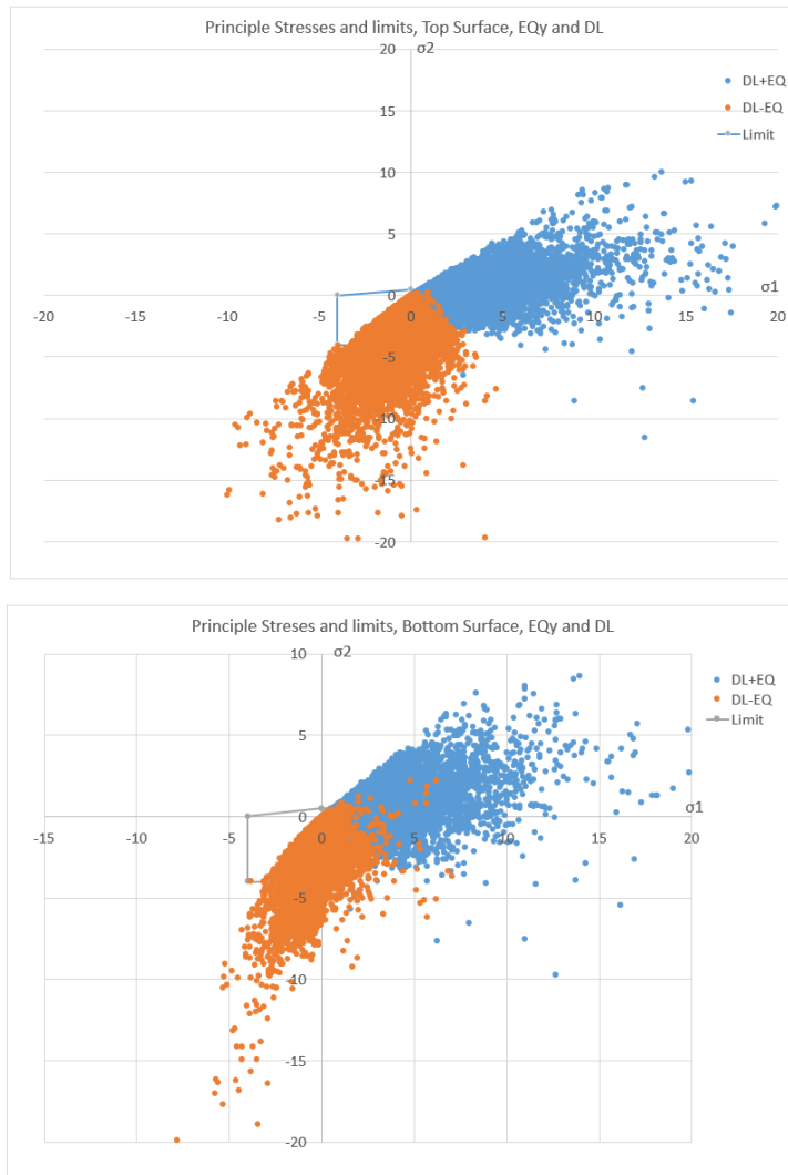
Figure 3.34. Limits of principle stresses using Coulomb-Mohr Theory
