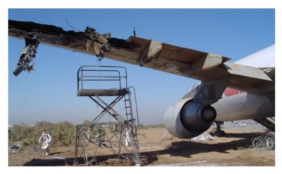
Figure 1.1: The Photo of Airbus A300B4-203(F) hit by missile, flight OO-DLL [9].
