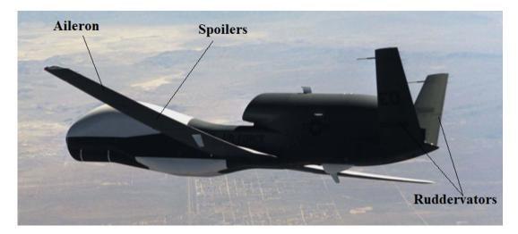
Figure A.2: Global Hawk UAV Flight Controls [15].
