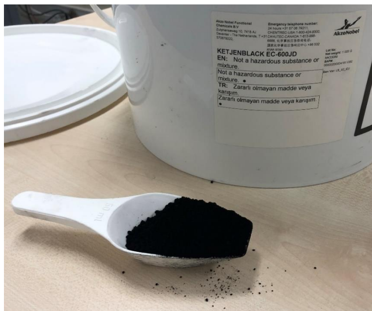
Figure 5-6 Ketjenblack aggregated dust particles
