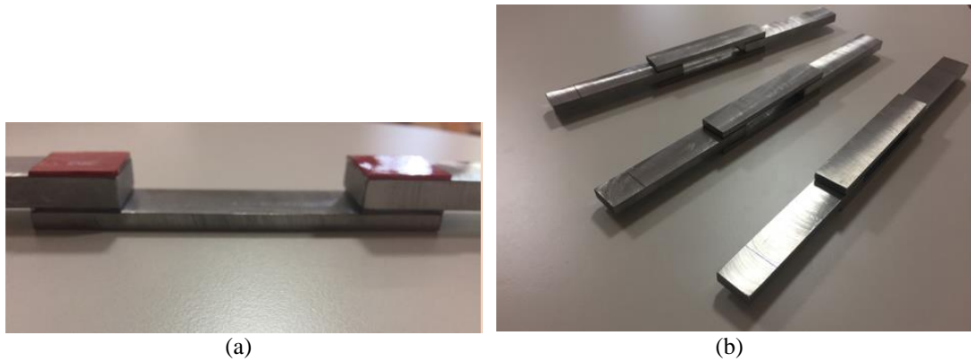
Figure 4-16 Bonding for quad lap shear test (a) Bonding step (b) Completed test apparatus
