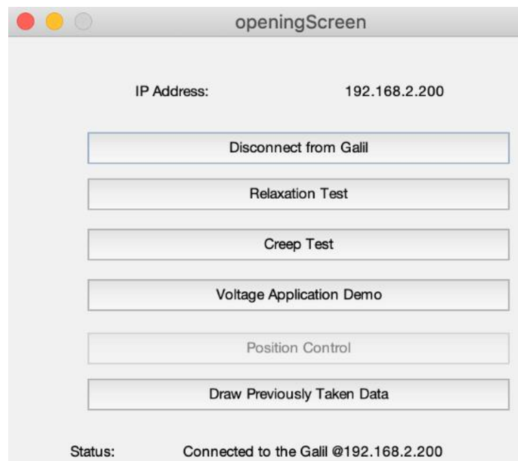
Figure 5-21 Matlab GUI opening screen to connect Galil controller
