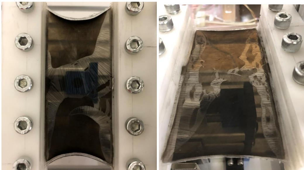
Figure 5-47 Face crimping failure mode
