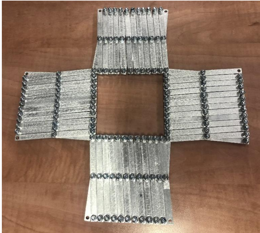
Figure 5-1 Prestretching scissor mechanism
