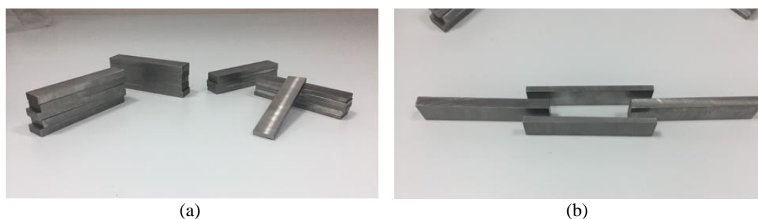
Figure 4-15 Text fixture preparation for quad lap shear test (a) Metal blocks (b) Test configuration
