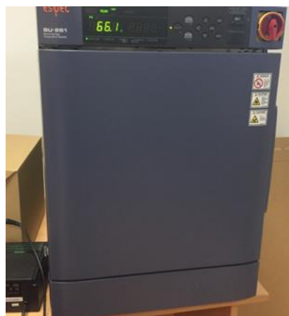
Figure 4-17 Heat chamber used to speed up bonding process
