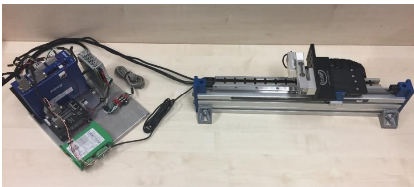
Figure 5-13 Linear translation stage and its controller unit
