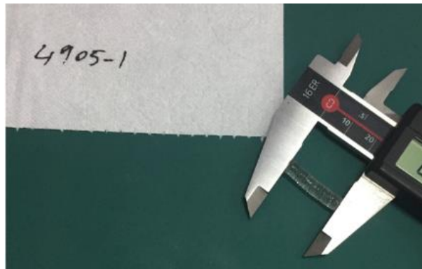
Figure 4-9 The Samples are removed from test fixture and then measured
