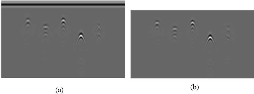
Figure 2.8. (a) Raw GPR Data, (b) Ground Bounce Removed GPR Data
