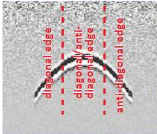
Figure 2.22. Diagonal Edge / Both Diagonal and Anti-Diagonal Edges / Antidiagonal Edge Regions
