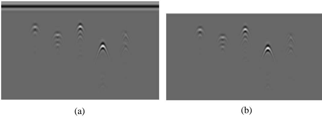
Figure 3.9. (a) Raw GPR Data, (b) Ground Bounce Removed GPR Data
