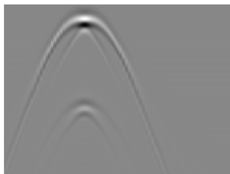
Figure 2.18. Ground Bounce Removed Raw Image
