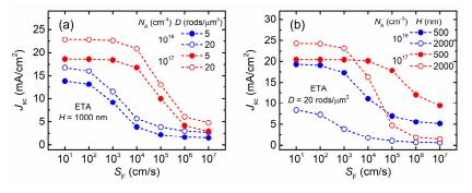
Fig. 7. Effect of CdS/CdTe surface recombination velocity on the  $J_{sc}$  for ETA cells with (a) 1000 nm-tall and 5 rods/ $\mu$ m<sup>2</sup>- and 20 rods/ $\mu$ m<sup>2</sup>-dense NRs, and (b) 500 nm- and 2000 nm-tall and 20 rods/ $\mu$ m<sup>2</sup>-dense NRs.
