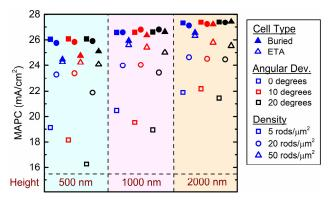
Fig. 2. The MAPC of ETA and buried cells for various heights, angular deviations and densities of ZnO NRs.
