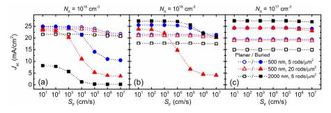
Fig. 6. Effect of surface recombination velocity at the CdS/CdTe interface on the  $J_{sc}$  for buried cells with 500 nm-tall and 5 rods/ $\mu$ m<sup>2</sup>, 500 nm-tall and 20 rods/ $\mu$ m<sup>2</sup>, and 2000 nm-tall and 5 rods/ $\mu$ m<sup>2</sup>-dense NRs and planar cells with same equivalent thicknesses for  $N_A$  of (a) 10<sup>15</sup> cm<sup>-3</sup>, (b) 10<sup>16</sup> cm<sup>-3</sup> and (c) 10<sup>17</sup> cm<sup>-3</sup>.
