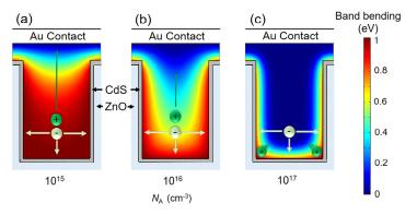
Fig. 5. Band bending in CdTe layer of buried cells with 500 nm-tall and 20 rods/ $\mu$ m<sup>2</sup>-dense NRs for  $N_A$  of (a) 10<sup>15</sup>, (b) 10<sup>16</sup> and (c) 10<sup>17</sup> cm<sup>-3</sup>. White and green arrows demonstrate the tentative paths of electrons and holes, respectively. White and green circles represent electrons and holes, respectively.
