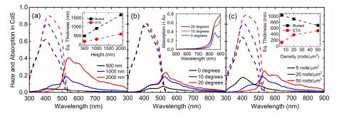
Fig. 3. The absorption spectra of CdS (dashed lines) and haze spectra of ZnO/CdS NRs in the absence of CdTe and Au layers (solid lines) at various (a) NR heights for an angular deviation of 10° and a 20 rods/ $\mu$ m<sup>2</sup> density, (b) angular deviations for a height of 1000 nm and a 20 rods/ $\mu$ m<sup>2</sup> density and (c) NR densities for a height of 1000 nm and an angular deviation of 10°.
