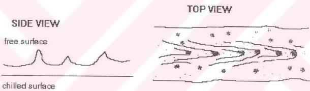
Figure 4.9 Flow pattern of free surface of a ribbon showing accumulated particles and elliptical lines along its entire length. It is obtained by PFC under the highest pressure (450 KPa) and the average thickness is noted as 250 mm.
