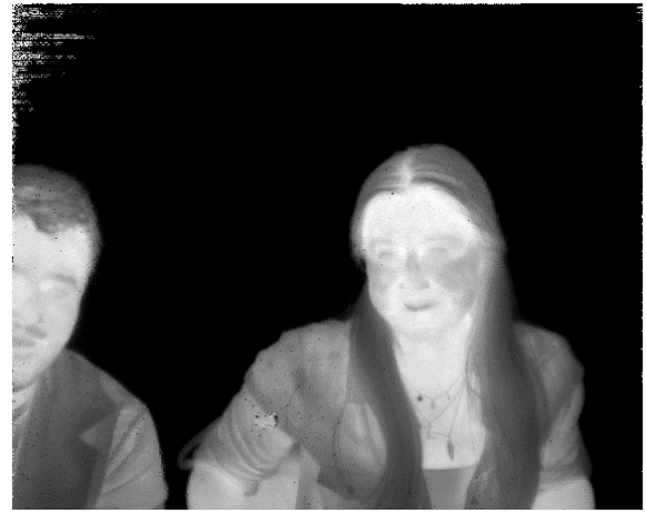
Fig. 9. An image acquired by FPA having a 50 \mu\text{m} thick substrate.
