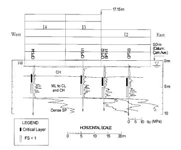
**Fig. 12.** West to east generalized soil profile of Site I (cross section A-A' in Fig. 11)
