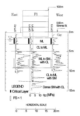
Fig. 9. East to west generalized subsurface soil profile of Site F
