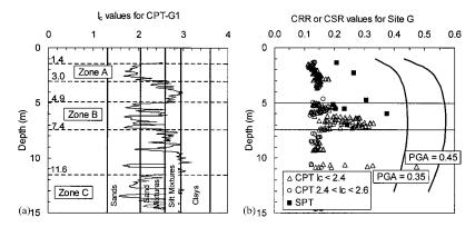
**Fig. 16.** Representative soil data for Site G: (a) Soil behavior index ( $I_c$ ) values for CPT-G1, and (b) cyclic stress ratio (CSR) induced by earthquake versus depth for peak ground acceleration (PGA)=0.35g and 0.45g compared with the cyclic resistance ratio (CRR) of the soil
