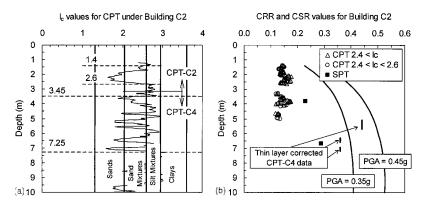
**Fig. 7.** (a) Soil behavior index ( $I_c$ ) values for CPT-C4 (Building C2), and (b) cyclic stress ratio (CSR) induced by the earthquake versus depth for free-field acceleration of 0.35g and 0.45g compared with the cyclic resistance ratio (CRR) of the soil for Building C2
