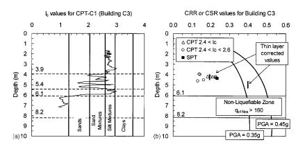
**Fig. 6.** (a) Soil behavior index ( $I_c$ ) values for CPT-C1 (Building C3), and (b) cyclic stress ratio (CSR) induced by the earthquake versus depth for free-field acceleration of 0.35g and 0.45g compared with the cyclic resistance ratio (CRR) of the soil for Building C3
