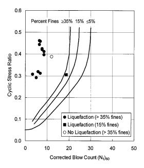
**Fig. 3.** Relationship between cyclic stress ratio and standard penetration test penetration resistance for sands and silty sands based on field performance data showing data for critical layers at selected sites in Adapazari [modified from Youd et al. (2001) after Seed et al. (1985)]
