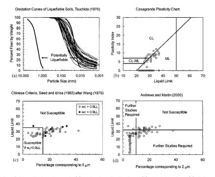
**Fig. 18.** Characteristics of liquefiable soils in Adapazari: (a) grain size distributions; (b) plasticity chart; (c) Chinese criteria for liquefaction of clayey soils after Seed and Idriss (1982) (after Wang 1979); and (d) liquefaction criteria for silty soils after Andrews and Martin (2000)
