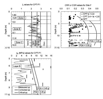
**Fig. 10.** Representative soil data for Building F: (a) Soil behavior index ( $I_c$ ) values for CPT-F1, (b) cyclic stress ratio (CSR) induced by earthquake versus depth for peak ground acceleration (PGA)=0.35g and 0.45g compared with the cyclic resistance ratio (CRR) of the soil, and (c) measured  $q_c$ , thin layer corrected  $q_c$ , and critical  $q_c$  for PGA=0.35g and 0.45g versus depth for Zone B
