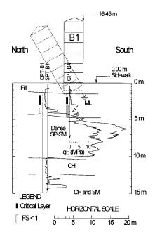
**Fig. 17.** Soil profile at Site B where a tall slender building failed in bearing
