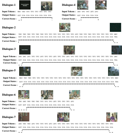
Figure 3: Dialogue scene analysis for MPEG-7 Test Data Set (CD-21) using a circular HMM (Ground truth is shown as a pulse diagram while dialogues are solid lines).
