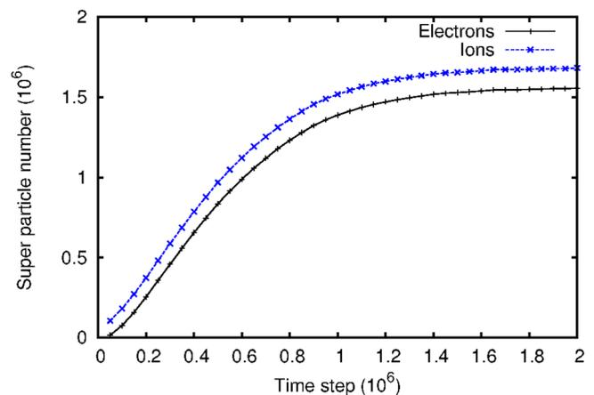
FIG. 4. Convergence test: number of super electrons and ions versus the time step. Conditions are given in Table III.
