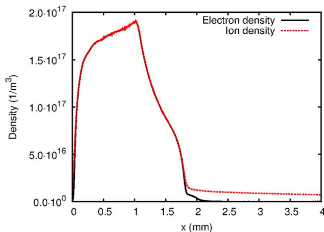
FIG. 7. Electron and helium ion density in the He-Ar mixture. Conditions are the same as in Fig. 5.
