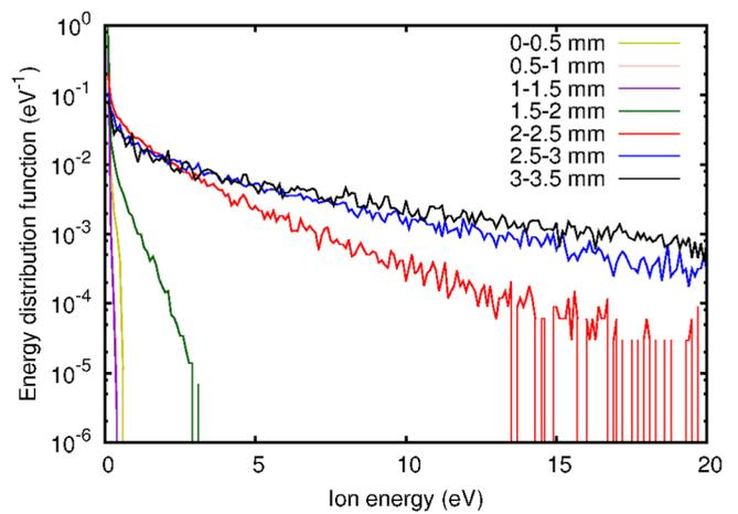
FIG. 8. Helium ion EDF's obtained in the He-Ar mixture. Conditions are the same as in Fig. 5.
