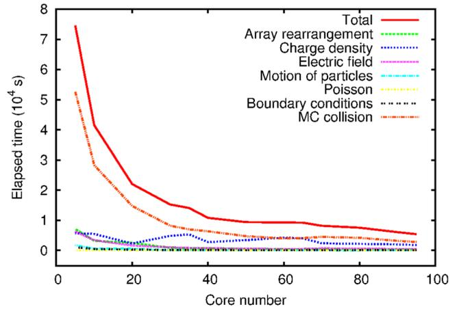
FIG. 3. Efficiency test for parallel PIC/MCC code. Results shown correspond to the range from 5 to 95 core numbers. Conditions are given in Table II.
