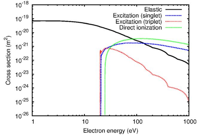
FIG. 1. Electron cross-sections for elastic, excitation, and direct ionization collisions in helium used in the model.<sup>16</sup>
