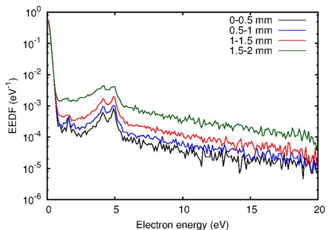
FIG. 9. EEDF's obtained in the He-Ar mixture. Conditions are the same as in Fig. 5.
