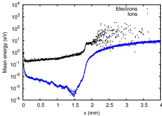
FIG. 6. Electron and helium ion mean energies in the He-Ar mixture.
