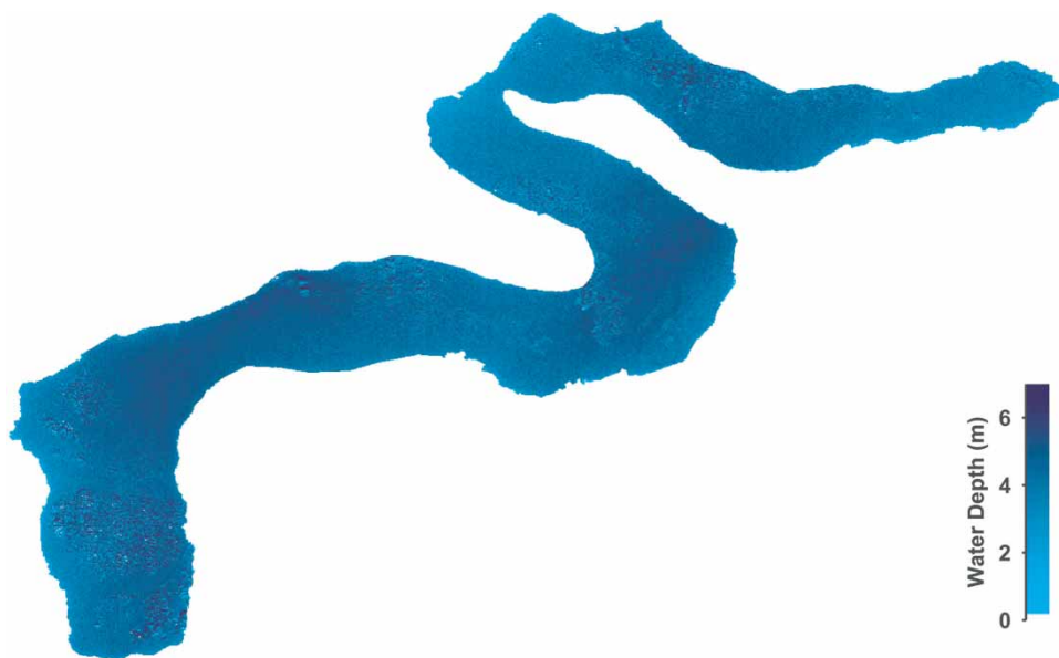
Figure 4 | The bathymetric map of Lake Eymir generated by the linear regression depth model.
