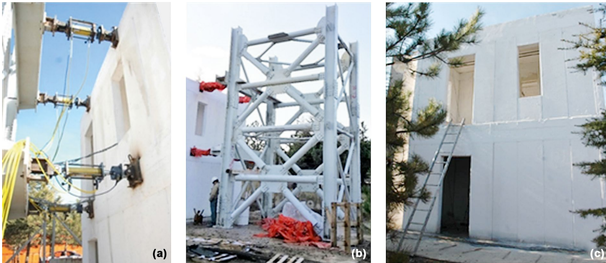
Fig. 2. Photographs of the test building and its loading system: (a) installed hydraulic actuators, (b) strong steel frame, and (c) the test building
