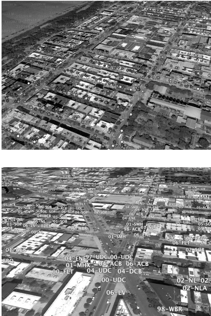
Figure 11 These are screenshots from the visualization module. In the upper plot, manholes are indicated by circles and shaded by vulnerability according to the predictive model. In the lower plot, geocoded locations of trouble tickets are indicated on the map, each labeled by trouble type and year.
