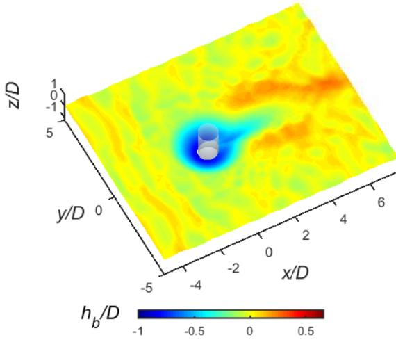
Figure 5: Equilibrium near-pile bed profile of Test 2
