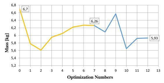
Figure 5.47: Combined optimization results for the Mesh 3 / Strength and local buckling constraints
