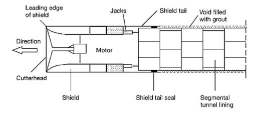
Figure 2.3. Typical Longitudinal Section of Tunnel Shield (Chapman et al., 2010)
