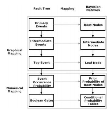
Figure 2.6. Mapping form FT to BN Model (Khakzad et al, 2011)
