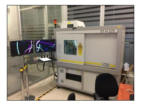
Figure 4: The core sample of the uppermost Bedinan Formation, 1<sup>st</sup> sandstone level from F well is used to determine pore type, volume, size and porosity via Nikon's XT H 225 X-ray computed tomography scanner.
