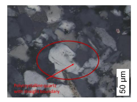
Figure 33: The photomicrograph of the core-1, the 1<sup>st</sup> sandstone level of the uppermost Bedinan Formation, F well, polycrystalline quartz with straight boundary.
