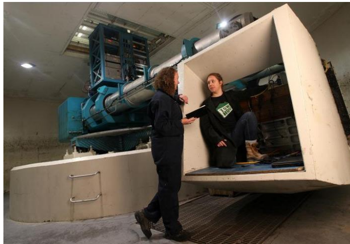
Figure 4.7. C-CORE's 5.5m-radius, 200g capacity Actidyn centrifuge (C-Core)
