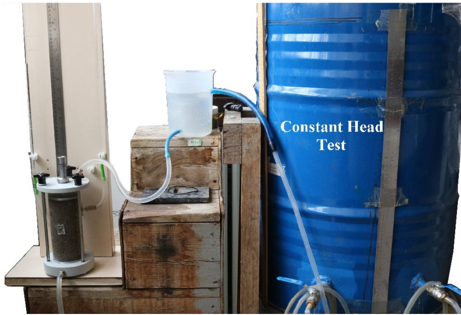
Figure 3.20. Determination of hydraulic conductivity of sand using constant head test
