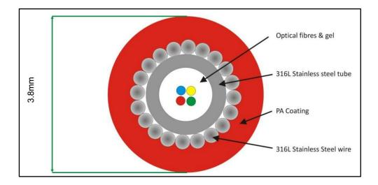
*Figure 4.10.* Inner layers of the Silixa multi-mode single steel wall tube armoured fiber optic duplexed cable. Two duplex Fiber cores and outer layers of the fiber.
