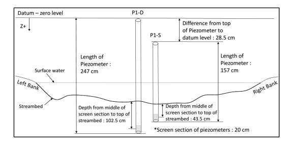
Figure 4.15. A sketch for piezometers of location P1
