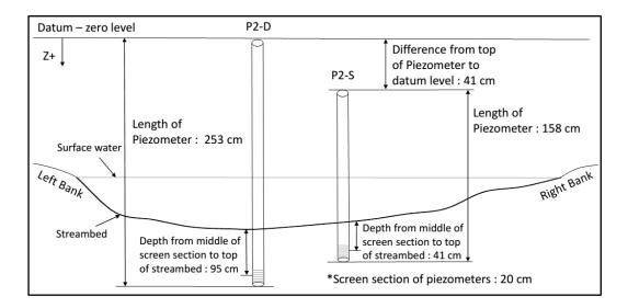
Figure 4.16. A sketch for piezometers of location P2
