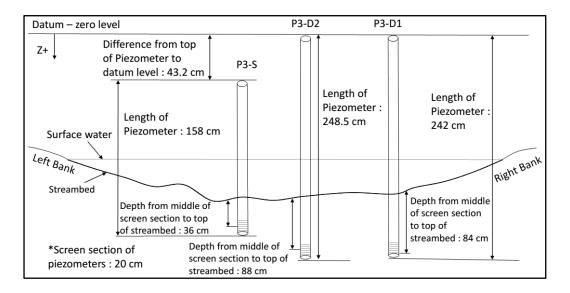
Figure 4.17. A sketch for piezometers of location P3
