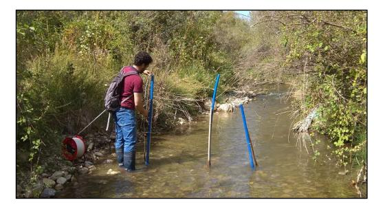
Figure 4.18. Water level, EC and temperature measurement using TLC meter
