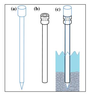
*Figure 4.14.* Installation units; (a) Metal pointed inner driver rod, (b) Outer metal tube that prevents collapse of opening during installation of piezometer, and (c) driving in installation units into streambed.
