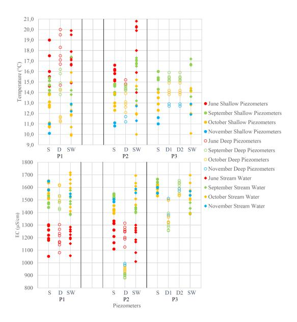
*Figure 5.21.* EC (25 °C) and temperature measurements from piezometers and stream water
