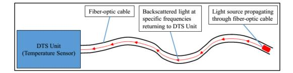
Figure 2.5. Illustration of fiber-optic distributed temperature sensing technology
