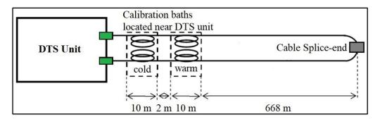
*Figure 4.12.* Field setting of FO-DTS system and length of the cables (adapted from Van de Giesen et al., 2012)
