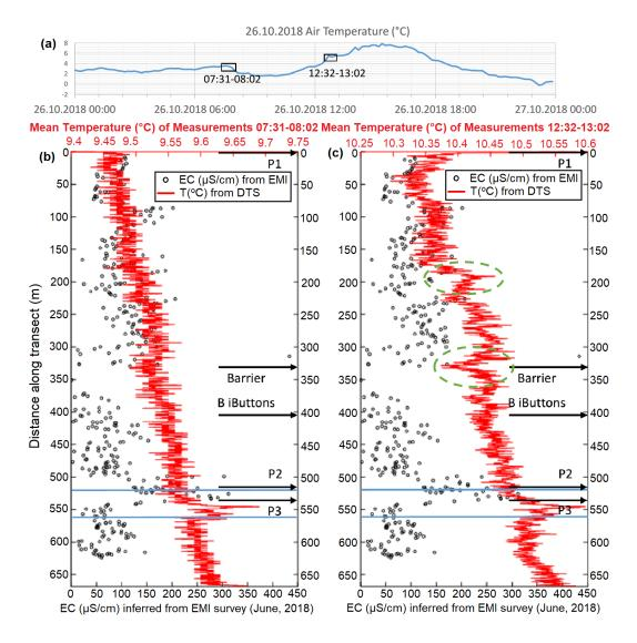
*Figure 5.12.* (a) air temperature, and EC data inferred from EMI Survey (June, 2018) overlain by mean top-of-the-streambed temperature values measured by the DTS unit on 26.10.2018 (b) at 07:31-08:02, and (c) at 12:32-13:02. Green circles in (c) indicate the effect of sunlight and shading which are not present in (b).
