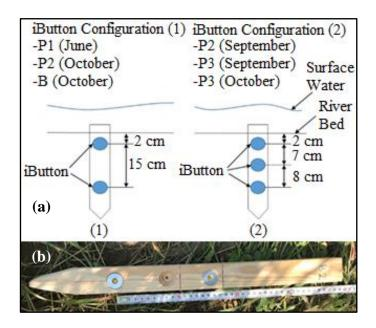
*Figure 4.19.* (a) Configurations of iButton Thermochrons at each location, (b) photo showing the configuration at location P1 in June field trip.
