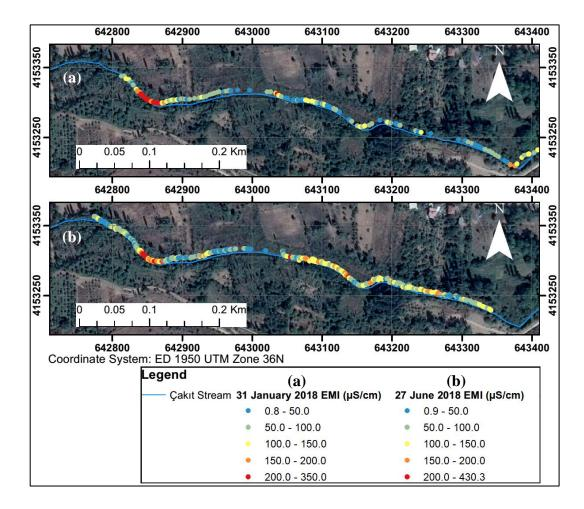
*Figure 5.2.* EC values (µS/cm) of streambed sediments inferred from EMI surveys on (a) 31 January, 2018, and on (b) 27 June, 2018
