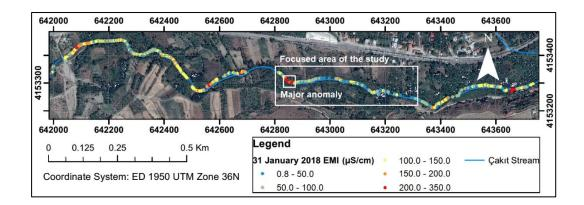
*Figure 5.1.* EC values (µS/cm) of streambed sediments inferred from EMI Survey performed on 31 January, 2018
