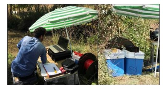
*Figure 4.13.* (a) A view of the field setup for the FO-DTS system and (b) calibration baths located near FO-DTS
