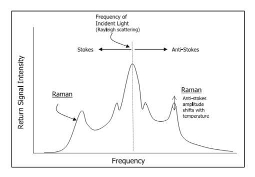
*Figure 2.6.* Raman backscattering of an incident light frequency (Adapted from Selker et al., 2006a)
