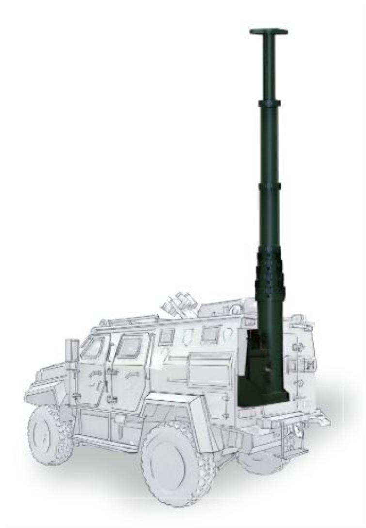
Figure 1.1: Illustration of the mast on an armoured vehicle, retrieved from [5]
