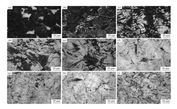
*Figure 2-2. Microstructures of 52CrMoV4 steel for different cooling rates a) 0.05 °C/sec b) 0.2 °C/sec c) 0.5 °C/sec d) 0.8 °C/sec e) 1 °C/sec f) 1.5 °C/sec g) 2 °C/sec h) 3 °C/sec i) 5 °C/sec [6]*
