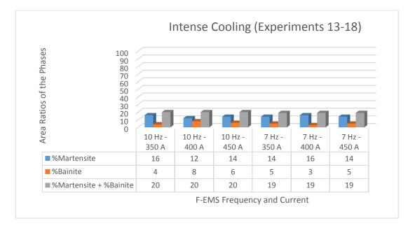
Figure 4-23. The area ratio of the phases for intense cooling experiments
