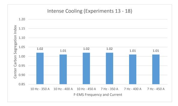
Figure 4-11. Center carbon segregation indexes for experiments with intense secondary cooling
