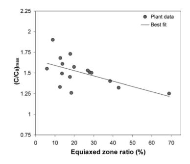
Figure 2-7. Variation of maximum degree of center carbon segregation index with equiaxed zone ratio [14]
