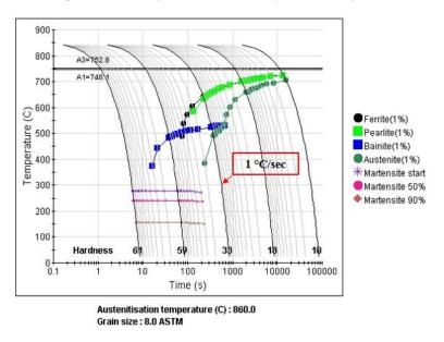
Figure 4-5. CCT of Site 3 calculated by JMatPro software
