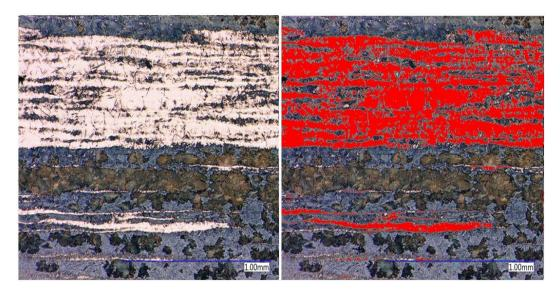
*Figure C-4. Microstructure of Experiment 4 (200X, 4% Picral, 60 sec.) and area ratio analysis* Image analysis show that the area ratio of the martensite phase (red region) is 37% and bainite (black region) is 36%.
