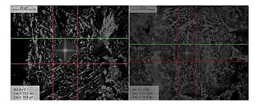
Figure 4-27. Micro hardness measurements on pearlite (353 HV 0.1 and 361 HV 0.05)
