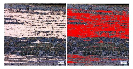
*Figure C-1. Microstructure of Experiment 1 (200X, 4% Picral, 60 sec.) and area ratio analysis* Image analysis show that the area ratio of the martensite phase (red region) is 39% and bainite (black region) is 37%.
