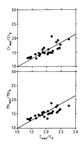
Figure 2-20. The relationship between center segregation indexes of carbon, chromium and manganese [38]
