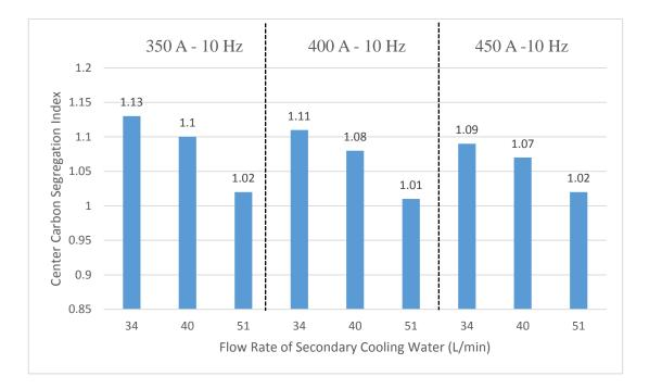
Figure 4-13. The effect of cooling intensity on center carbon segregation index
