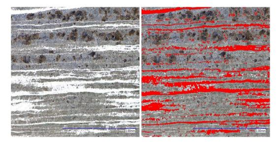
*Figure C-9. Microstructure of Experiment 9 (200X, 4% Picral, 60 sec.) and area ratio analysis* Image analysis show that the area ratio of the martensite phase (red region) is 26% and bainite (black region) is 18%.
