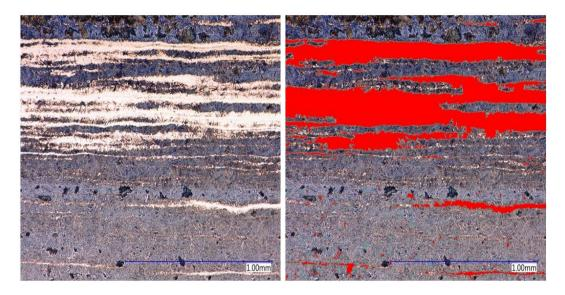
*Figure C-8. Microstructure of Experiment 8 (200X, 4% Picral, 60 sec.) and area ratio analysis* Image analysis show that the area ratio of the martensite phase (red region) is 29% and bainite (black region) is 8%.
