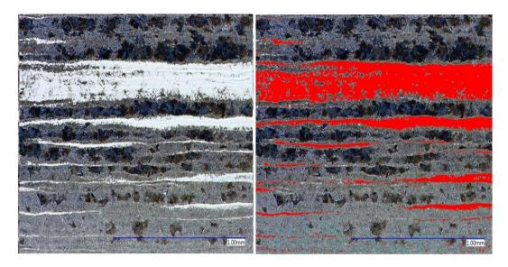
*Figure C-12. Microstructure of Experiment 12 (200X, 4% Picral, 60 sec.) and area ratio analysis* Image analysis show that the area ratio of the martensite phase (red region) is 25% and bainite (black region) is 26%.
