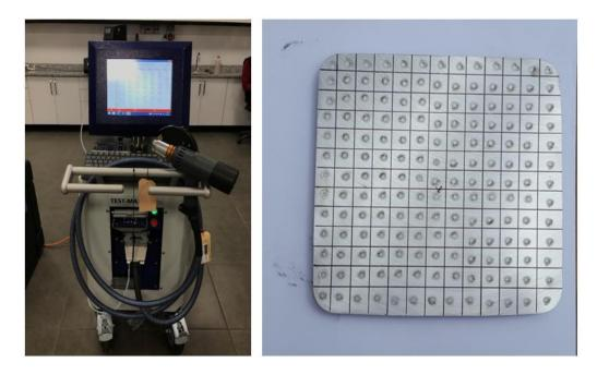
Figure 3-1. Test Master Pro mobile spectrometer and chemical composition measurements on transverse billet slice
