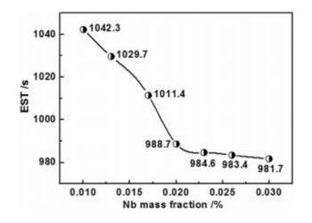
Figure 2-9. EST (sec) with different mass fractions of Nb (%) [19]
