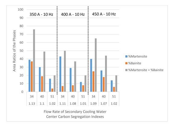
Figure 4-24. The effect of flow rate of secondary cooling water on microstructural banding intensity
