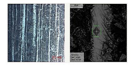
Figure 1-2. Microstructure of the sample taken from center of the product (LM, Nital, 15 seconds, 100X) and micro hardness measurement on white band (737 HV 0.1)
