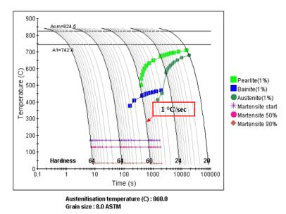
Figure 4-4. CCT of Site 2 calculated by JMatPro software
