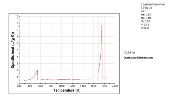
Figure 4-6. Specific heat of 52CrMoV4 steel at various temperatures
