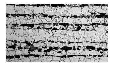
Figure 2-1. Ferrite-pearlite banding in a wrought 1018 steels (Nital, LM, 100X) [1]
