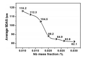
Figure 2-10. Average SDAS (µm) with different mass fractions of Nb (%) [19]
