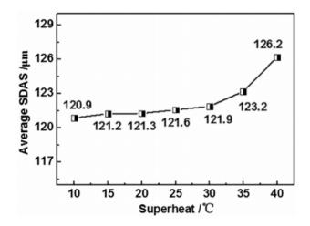
Figure 2-14. SDAS (µm) with different superheat [19]
