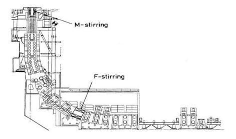
Figure 2-17. Position of M-EMS and F-EMS on a CCM [30]
