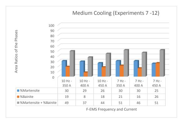
Figure 4-22. The area ratio of the phases for medium cooling experiments
