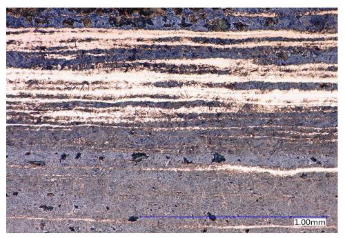
Figure 4-18. Microstructure of Experiment 8 having the lowest banding intensity among the medium cooling experiments (200X, 4% Picral, 60 sec.)
