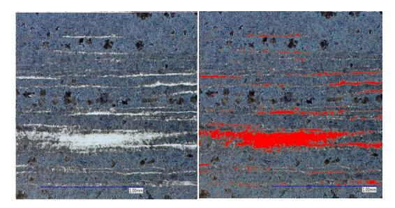
*Figure C-15. Microstructure of Experiment 15 (200X, 4% Picral, 60 sec.) and area ratio analysis* Image analysis show that the area ratio of the martensite phase (red region) is 14% and bainite (black region) is 6%.
