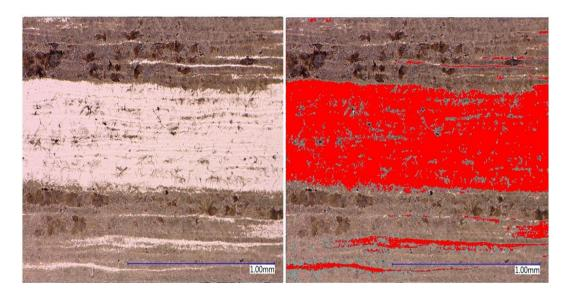
*Figure C-5. Microstructure of Experiment 5 (200X, 4% Picral, 60 sec.) and area ratio analysis* Image analysis show that the area ratio of the martensite phase (red region) is 43% and bainite (black region) is 11%.
