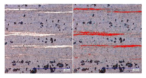
*Figure C-14. Microstructure of Experiment 14 (200X, 4% Picral, 60 sec.) and area ratio analysis* Image analysis show that the area ratio of the martensite phase (red region) is 12% and bainite (black region) is 8%.
