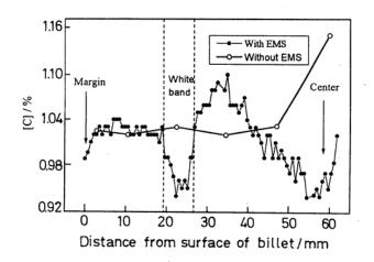
Figure 2-18. Carbon distribution in 120x120 mm billets with and without EMS [34]
