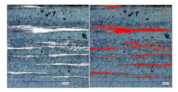
*Figure C-17. Microstructure of Experiment 17 (200X, 4% Picral, 60 sec.) and area ratio analysis* Image analysis show that the area ratio of the martensite phase (red region) is 16% and bainite (black region) is 3%.
