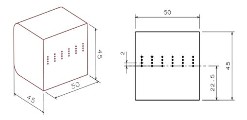
Figure 3-4. Hardness measurement points
