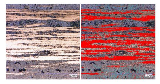
*Figure C-2. Microstructure of Experiment 2 (200X, 4% Picral, 60 sec.) and area ratio analysis* Image analysis show that the area ratio of the martensite phase (red region) is 43% and bainite (black region) is 7%.
