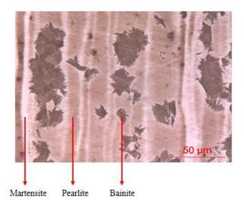
Figure 4-1. Microstructure of the sample taken from center of the plate product, 52CrMoV4, 90x45 mm (LM, LePera, 4 minutes, 100X)
