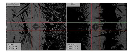
Figure 4-25.Micro hardness measurements on martensite bands (843 HV 0.1 and 788 HV 0.1)
