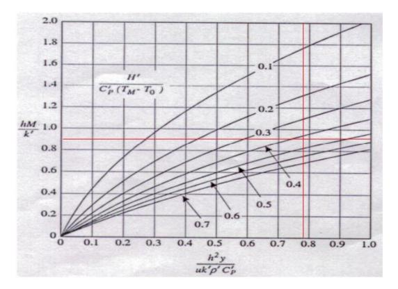
*Figure 4-8. Thickness solidified, M, versus distance down the mould [44]*
