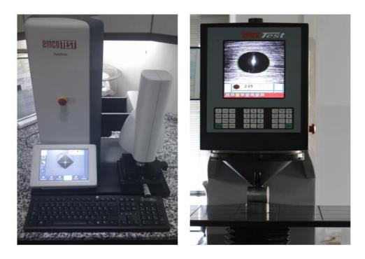
Figure 3-3. Emco Test Durascan 20 micro hardness test device and Emco Test M5C hardness test device
