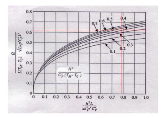
Figure 4-7. Rate of heat removal by mould cooling water versus mould length [44]
