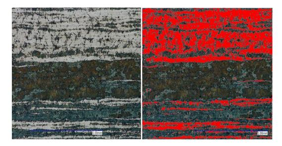
*Figure C-3. Microstructure of Experiment 3 (200X, 4% Picral, 60 sec.) and area ratio analysis* Image analysis show that the area ratio of the martensite phase (red region) is 40% and bainite (black region) is 25%.
