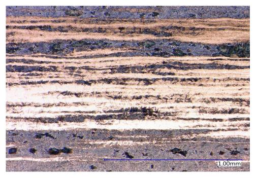
Figure 4-16. Microstructure of Experiment 2 having the lowest banding intensity among the mild cooling experiments (200X, 4% Picral, 60 sec.)
