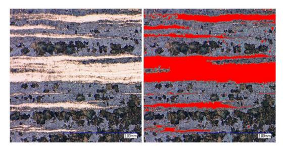
*Figure C-10. Microstructure of Experiment 10 (200X, 4% Picral, 60 sec.) and area ratio analysis* Image analysis show that the area ratio of the martensite phase (red region) is 30% and bainite (black region) is 21%.
