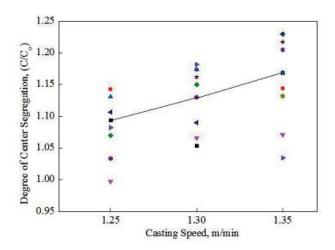
Figure 2-13. The effect of casting speed (strand velocity) on the degree of center segregation for carbon [25]
