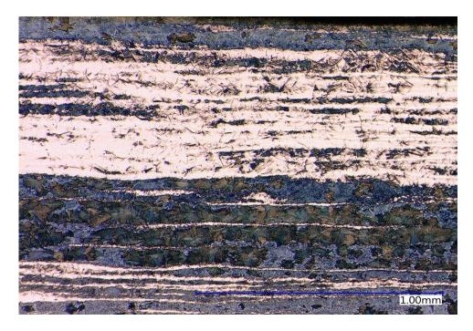
Figure 4-15. Microstructure of Experiment 1 having the highest banding intensity among the mild cooling experiments (200X, 4% Picral, 60 sec.)
