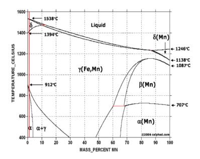
Figure 2-3. The Fe-Mn phase diagram [10]
