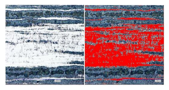
*Figure C-6. Microstructure of Experiment 6 (200X, 4% Picral, 60 sec.) and area ratio analysis* Image analysis show that the area ratio of the martensite phase (red region) is 43% and bainite (black region) is 16%.
