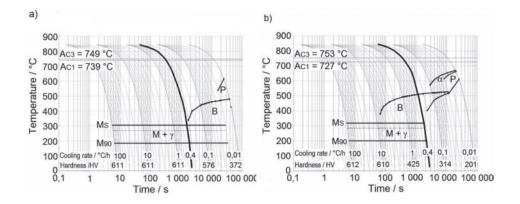
Figure 2-5. CCT diagrams of a) Site 1 and b) Site 2 [4]
