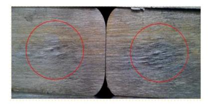
Figure 1-1. Uneven cutting surface of the plate products after cold sawing, 52CrMoV4, 90x45 mm
