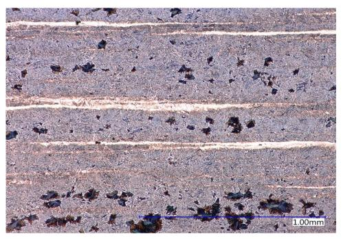
Figure 4-20. Microstructure of Experiment 14 having the lowest banding intensity among the intense cooling experiments (200X, 4% Picral, 60 sec.)
