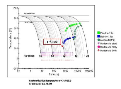
Figure 4-3. CCT of Site 1 calculated by JMatPro software
