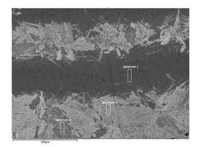
Figure 4-2. SEM micrograph of banded microstructure of 52CrMoV4 steel
