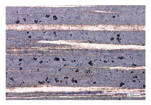
Figure 4-19. Microstructure of Experiment 13 having the highest banding intensity among the intense cooling experiments (200X, 4% Picral, 60 sec.)
