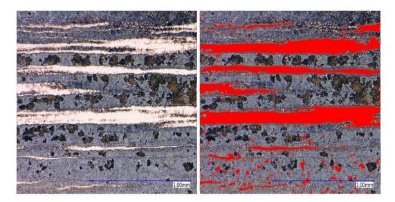
*Figure C-11. Microstructure of Experiment 11 (200X, 4% Picral, 60 sec.) and area ratio analysis* Image analysis show that the area ratio of the martensite phase (red region) is 30% and bainite (black region) is 16%.
