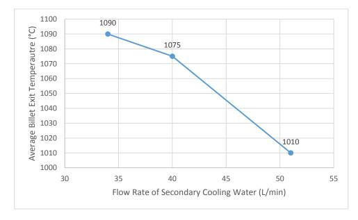
Figure 4-12. Average billet exit temperatures for different flow rates of secondary cooling water
