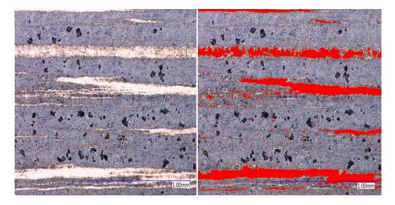
*Figure C-13. Microstructure of Experiment 13 (200X, 4% Picral, 60 sec.) and area ratio analysis* Image analysis show that the area ratio of the martensite phase (red region) is 16% and bainite (black region) is 4%.
