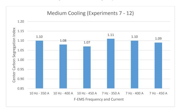
Figure 4-10. Center carbon segregation indexes for experiments with medium secondary cooling
