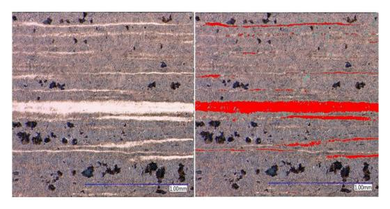
*Figure C-18. Microstructure of Experiment 18 (200X, 4% Picral, 60 sec.) and area ratio analysis* Image analysis show that the area ratio of the martensite phase (red region) is 14% and bainite (black region) is 5%.
