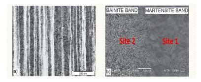
Figure 2-4. Banded microstructure in 34CrNiMo6 steel a) LM and b) SEM [4]
