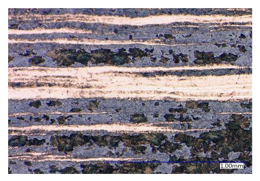
Figure 4-17. Microstructure of Experiment 10 having the highest banding intensity among the medium cooling experiments (200X, 4% Picral, 60 sec.)
