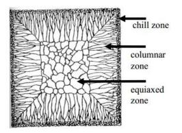
Figure 2-6. Sketch of continuous casting billet structure [13]
