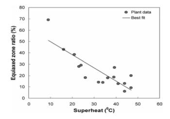
Figure 2-15. Variation of equiaxed zone ratio with the casting superheat [14]
