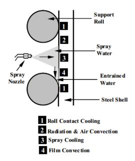
Figure 2-12. Different cooling mechanisms in the secondary cooling region [21]
