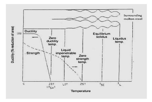
Figure 2-16. Mechanical properties of dendrites in mushy zone [28]
