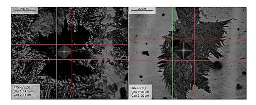
Figure 4-26. Micro hardness measurements on bainite (470 HV 0.05 and 464 HV 0.1)
