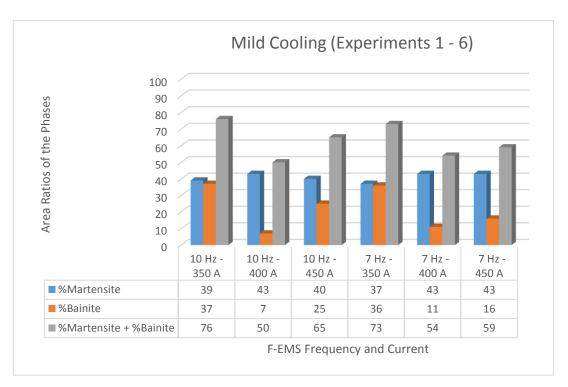
Figure 4-21. The area ratio of the phases for mild cooling experiments
