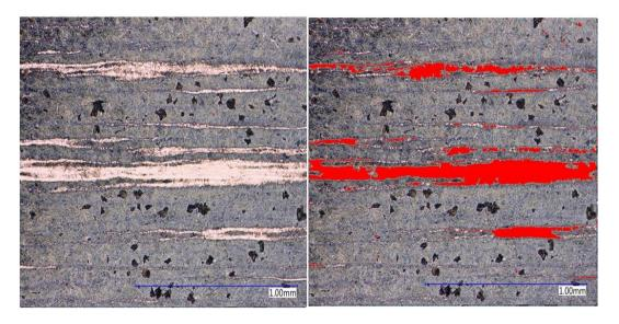
*Figure C-16. Microstructure of Experiment 16 (200X, 4% Picral, 60 sec.) and area ratio analysis* Image analysis show that the area ratio of the martensite phase (red region) is 14% and bainite (black region) is 5%.
