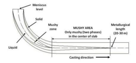
Figure 2-19. Sketch of inner structure of continuously casted billet [37]
