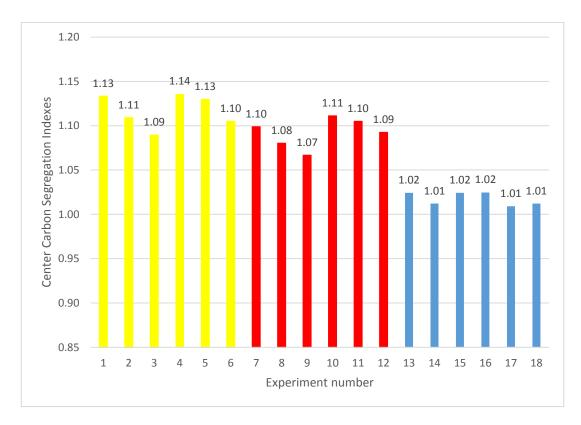
Figure 4-14. Center carbon segregation indexes for all experiments
