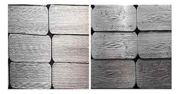
Figure 4-28. Comparison of cutting surfaces of the Experiment 14 (smooth) and Experiment 8 (uneven)
