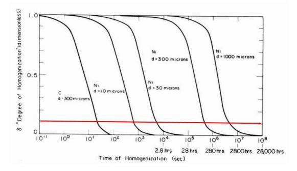
Figure 2-8. Degree of homogenization versus time at 1200 °C for nickel and carbon for different dendrite arm spacings [20]
