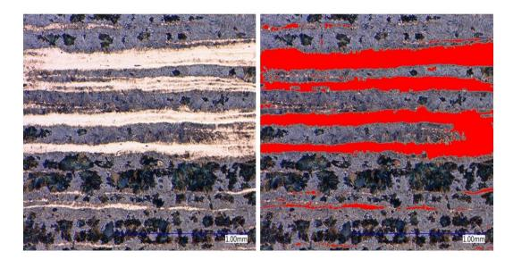
*Figure C-7. Microstructure of Experiment 7 (200X, 4% Picral, 60 sec.) and area ratio analysis* Image analysis show that the area ratio of the martensite phase (red region) is 30% and bainite (black region) is 19%.
