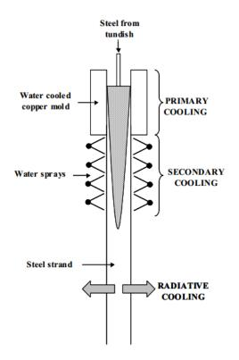
Figure 2-11. Schematic cooling process for continuous casting of steel [21]
