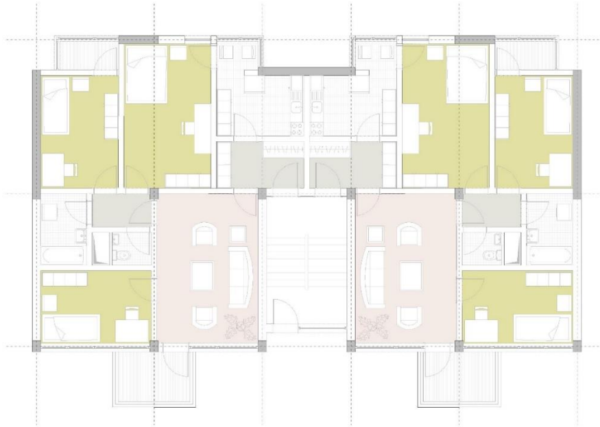
Figure 3.3. Architectural plan of a typical floor of first case study apartment building consisting of two flats
