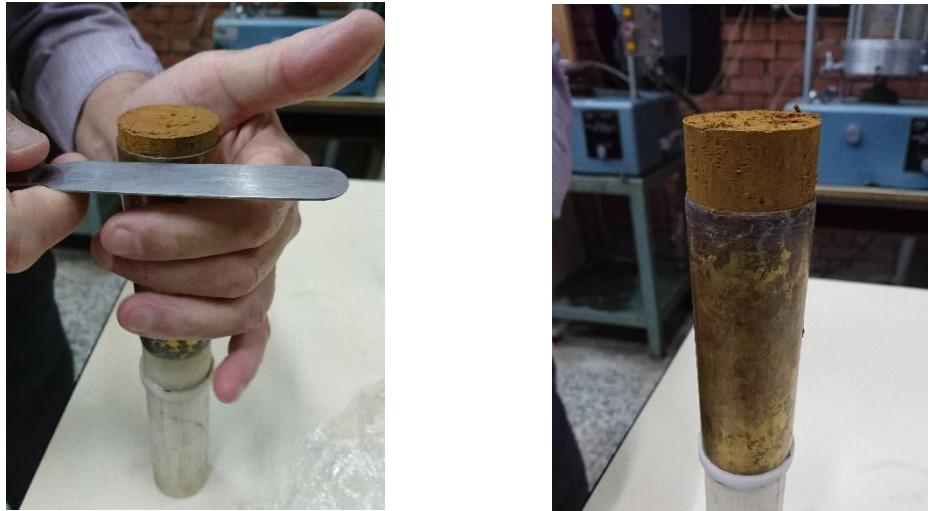
Figure 3.11. Specimen preparation for unconfined compression test from small tube samples
