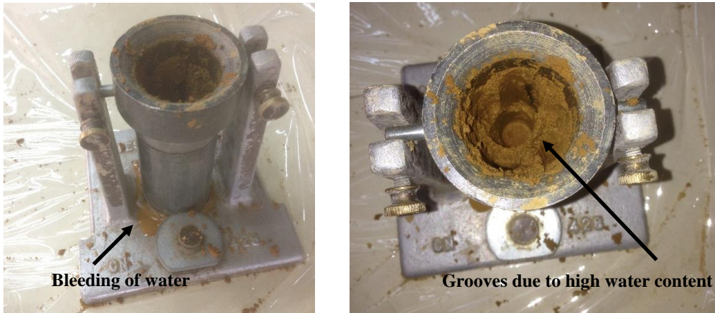
Figure 3.10. Encountered problems during Harvard compaction procedure
