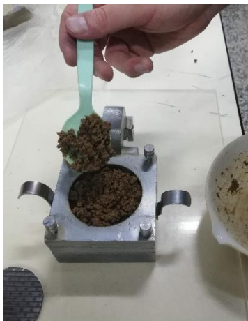
(a) soil placement for static compaction
