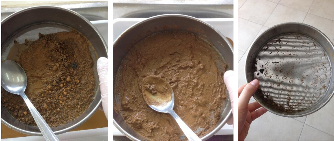
Figure 3.6. Soil wet sieving through 0.425 mm sieve
