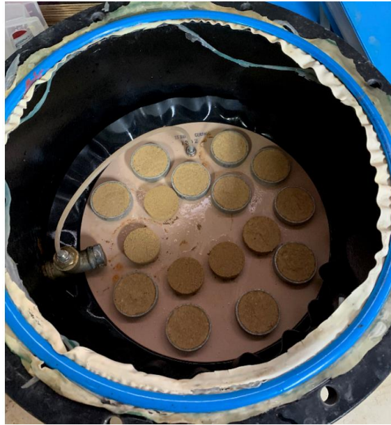
(b) Pressure plate apparatus (above the pressure plate soil specimens are shown)
