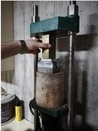
(c) soil compaction by hydraulic piston
