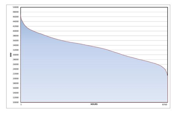
Figure 3.7. Load duration curve of 2017 [58]
