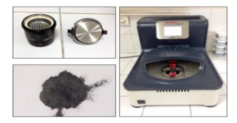
Figure 3.4 Fritsch Pulverisette 7 Premium Line High Energy Ball Mill, stainless steel bowl / balls and Ni-B powder mixture
