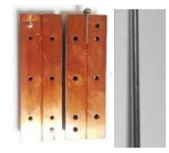
Figure 3.3 Copper mold and cylindrical Ni<sub>60</sub>B<sub>40</sub> bulk rod.
