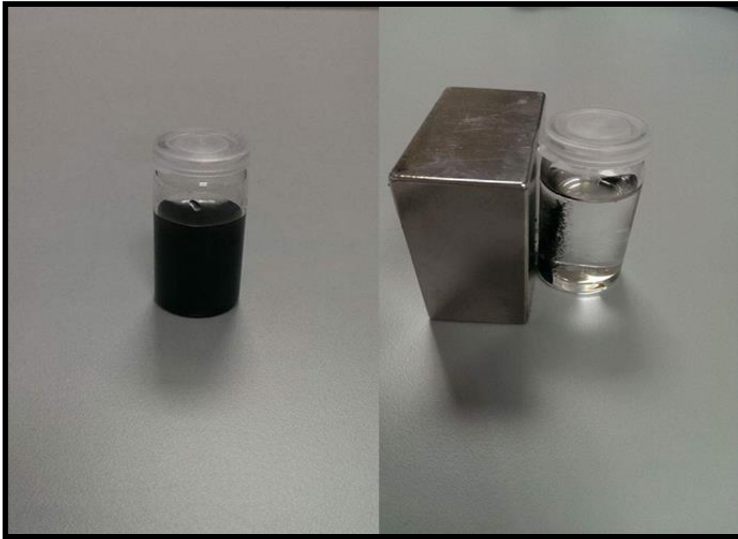
Figure 3.13. Magnetic behavior of MNP-PEDOT-TiO 2 composite material under externally applied magnetic field (1.6 T).
