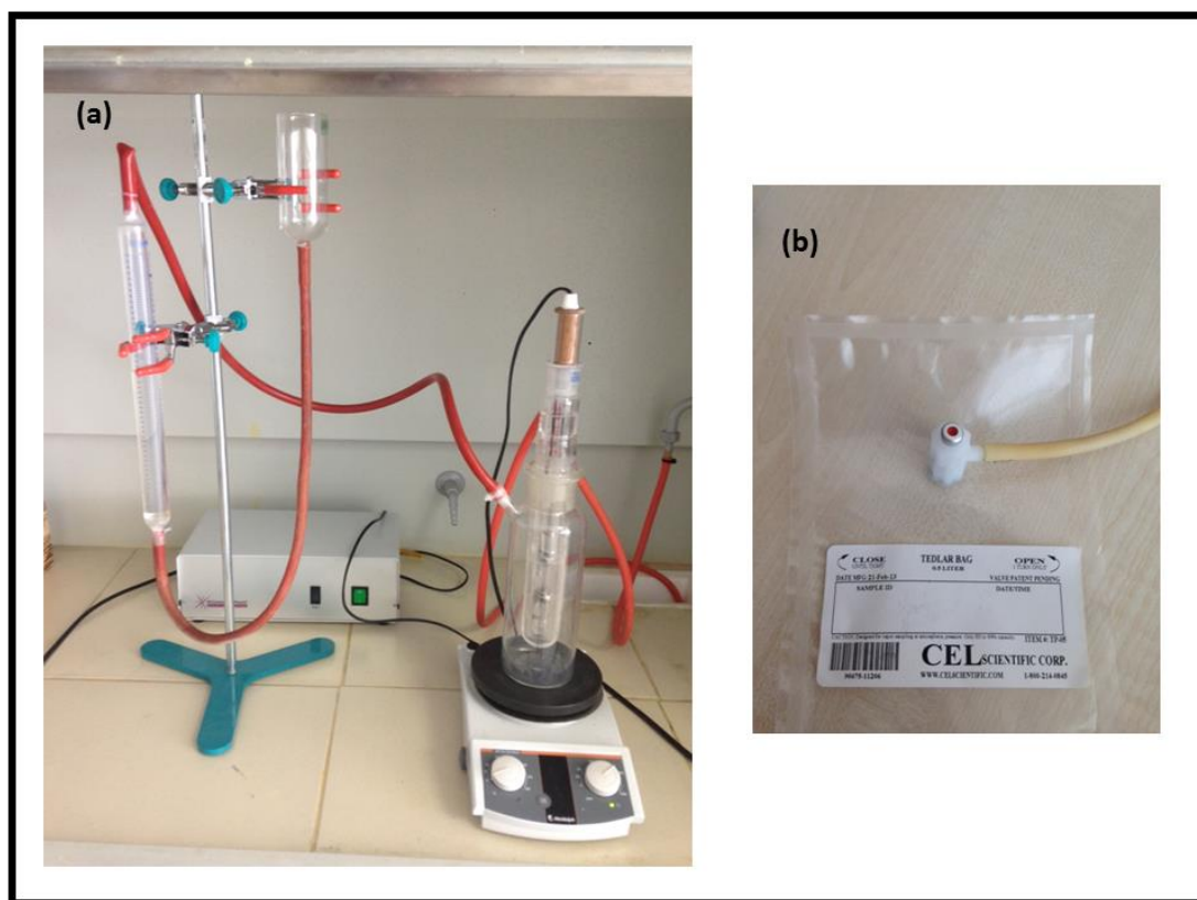
Figure 2.10. (a) System that was used to generate hydrogen gas from the ethanol-water mixture under UV light (b) Tedlar bag for collecting a gas sample for GC analyses.
