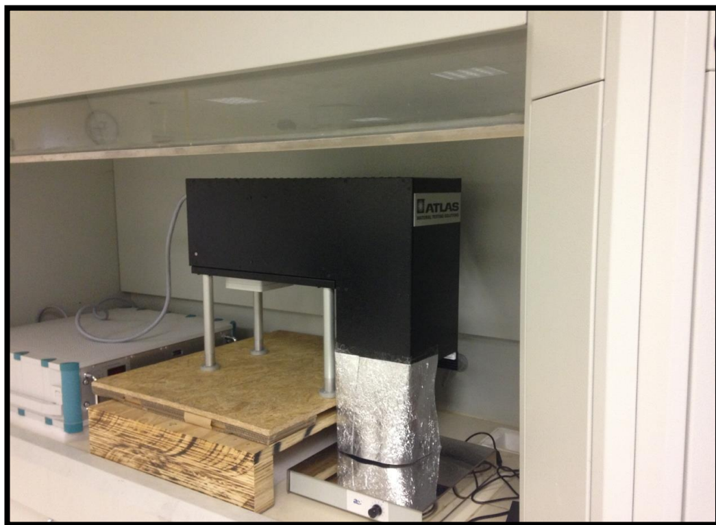
Figure 2.9. Atlas solar simulator system that was utilized throughout the photocatalytic efficiency tests.
