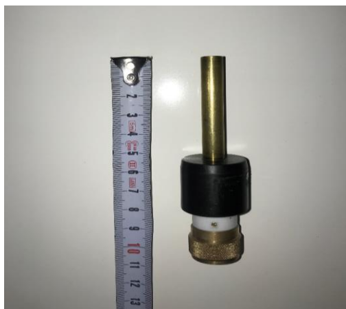
Figure 3.2. 10 cm-long monopole antenna
